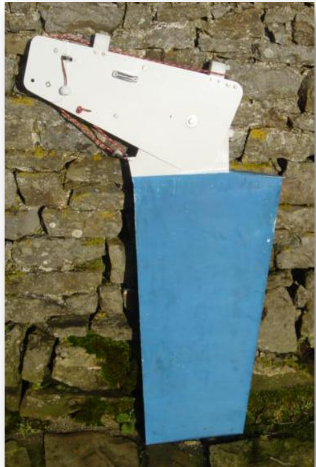
Lifting rudder showing rudder in the locked down & raised positions. The rudder is locked down by a stainless steel drop-head pin that passes through the rudder cheeks and the rudder blade.
