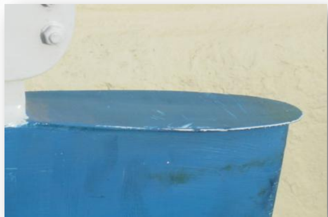
Lifting rudder showing rudder in the locked down & raised positions. The rudder is locked down by a stainless steel drop-head pin that passes through the rudder cheeks and the rudder blade.
