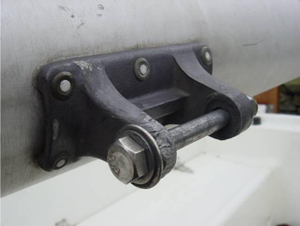
Gooseneck fitting – riveted to mast
