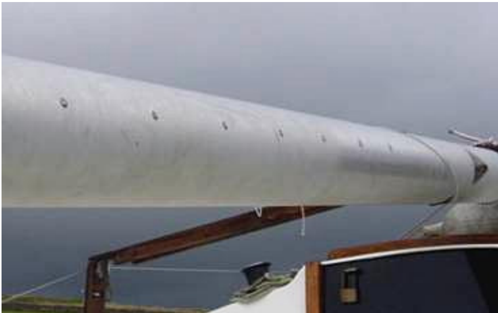
Rivet line along front face of mast
